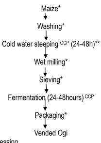
Figure 1: Flow diagram of *ogi* processing. Legend
