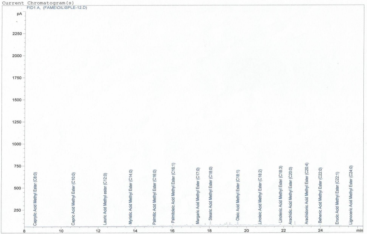
Fig.13: Chromatogram of sample degraded by Candida parapsilosis in medium 1 on the 10 th day of degradation.
