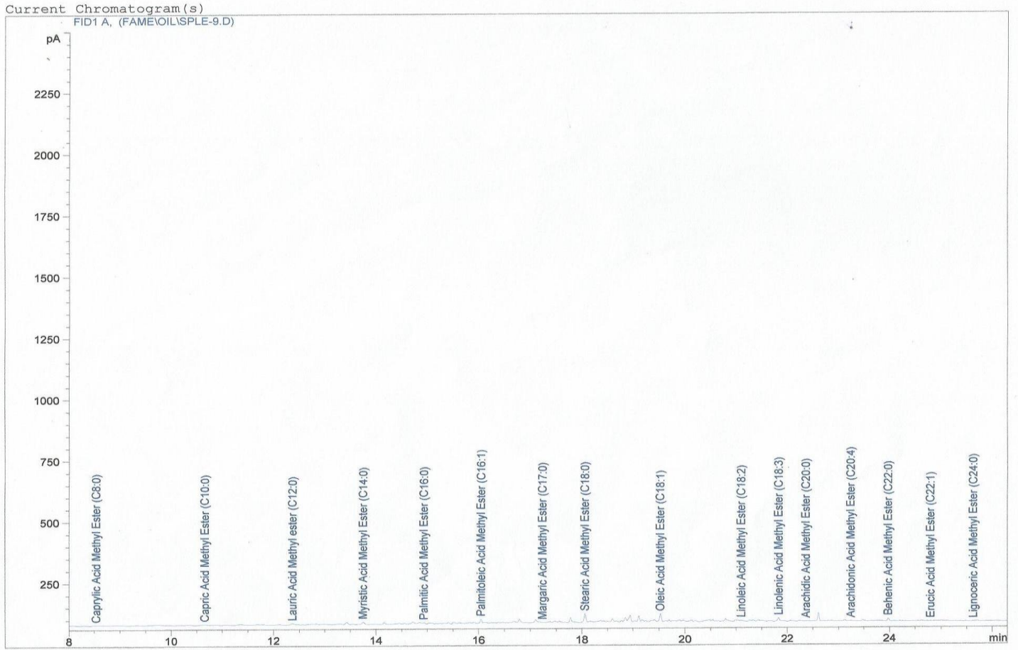
Fig.10: Chromatogram of sample degraded by Pseudomonas fluorescens in medium 2 on the 20 th day of degradation.
