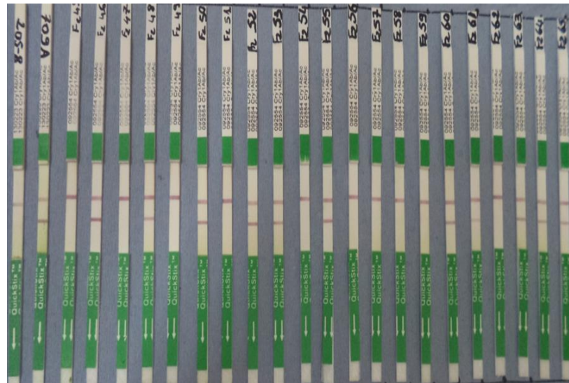
Two bands=presence of Bt protein; one band=absence of Bt protein Photo 3: ELISA test of F 2 offspring derived from IT98K-205-8 /709A
