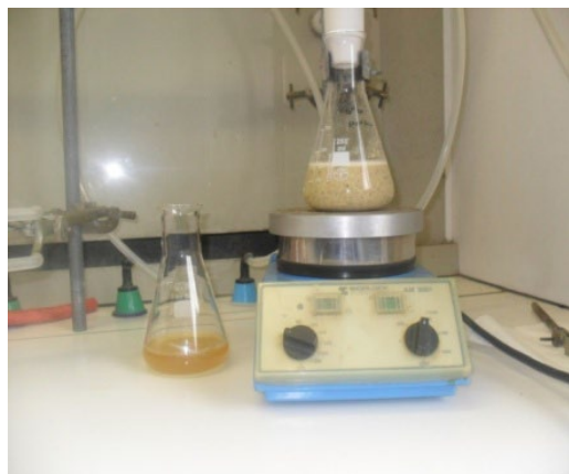
Figure 2 : montage extraction solide/liquide
