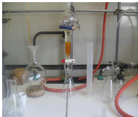
Figure 3: extraction liquide- liquide au
